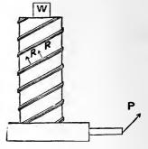
with it. The groove being supposed smooth, these reactions are at right angles to it.
